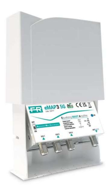
3-Input (VHF+DAB / UHF) smart self-programmable head-end for external polemounting installation, 32 high selectivity filters.
